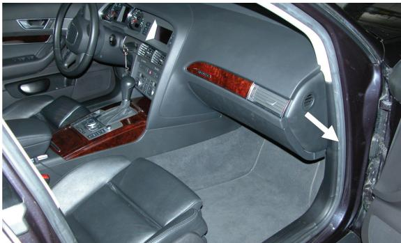
(EN) Filter is located behind the glove compartment. Remove the upholstery panel
